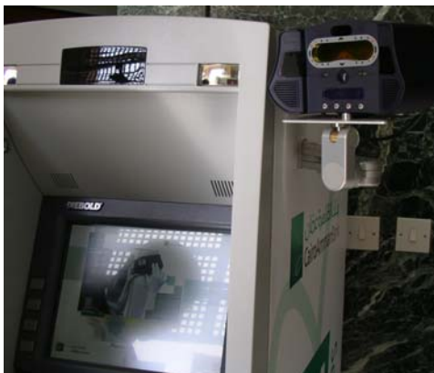
Banks in Jordan use iris recognition to verify customer identity (top right)
